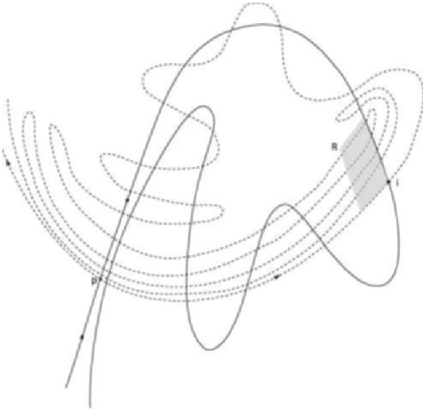
Fig. 17. Schematic representation of the stable and unstable manifolds W_u(p) and W_s(p) of a fixed point p , a homoclinic point r , and a small quadrilateral R in its neighborhood.
